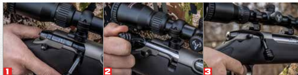
Position 1: Locks the bolt into safe
